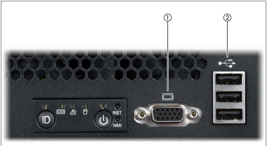
Figure 3: Connectors on the front
